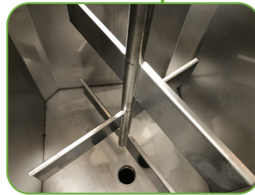
Laser cutting stainless steel SUS304 for Sludge water tank and Polymer mixing tank.
