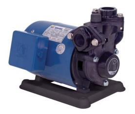
Power: 0.37 kW 50Hz Head: Up to 35 M Flow: Up to 35 L/min 60Hz Head: Up to 40 M Flow: Up to 42 L/min Outlet: 3/4" - 1"
