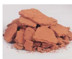
经脱水处理后形成泥饼状 The Slurry Cake after dehydrating.
